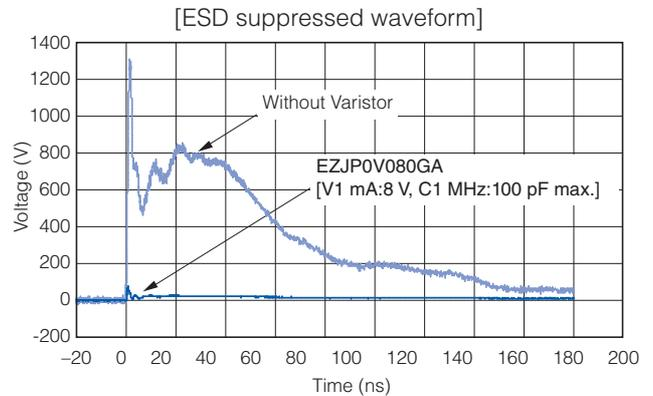
\* IEC61000-4-2 ... International Standard of the ESD testing method (HBM) for electronic equipment ability to withstand ESD generated from a human body. It sets 4 levels of severity
