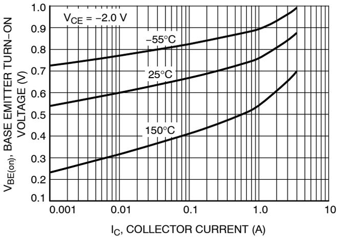
Figure 5. Base Emitter Turn-On Voltage vs. Collector Current
