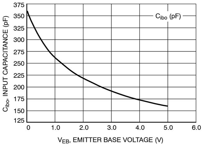
**Figure 7. Input Capacitance**
