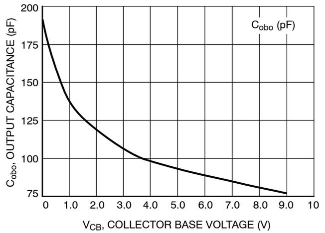
**Figure 8. Output Capacitance**
