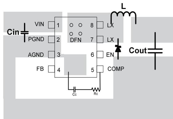
Figure 4. AOZ1094 (DFN-8) PCB Layout
