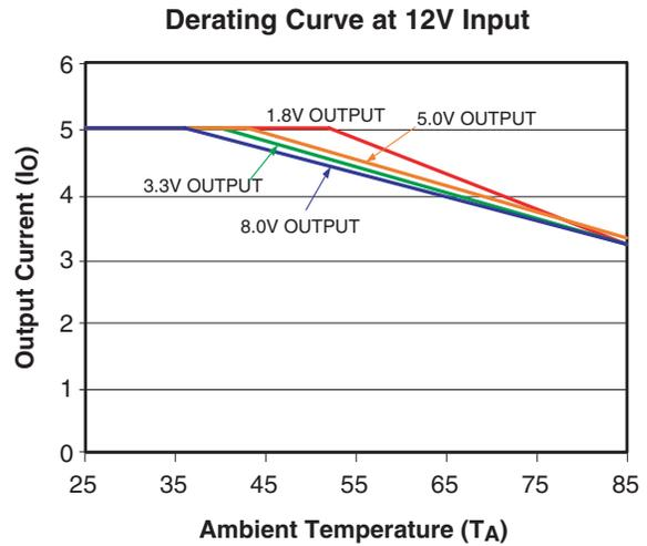
Thermal de-rating curves for DFN-8 package part under typical input and output conditions. Circuit of Figure 1. 25°C ambient temperature and natural convection (air speed < 50LFM) unless otherwise specified.
