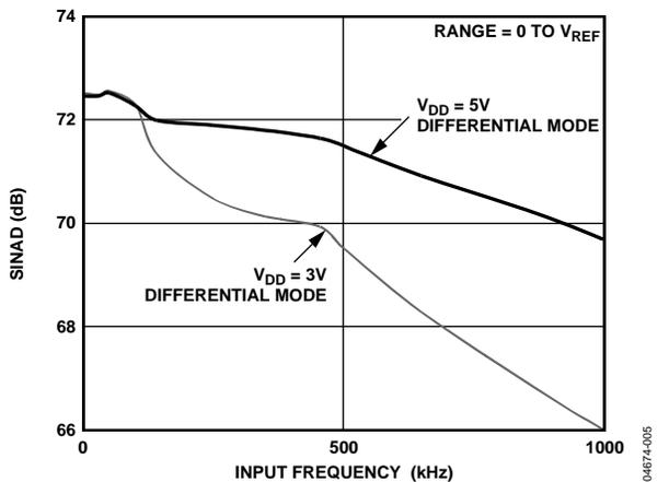
Figure 6. SINAD vs. Analog Input Frequency for Various Supply Voltages
