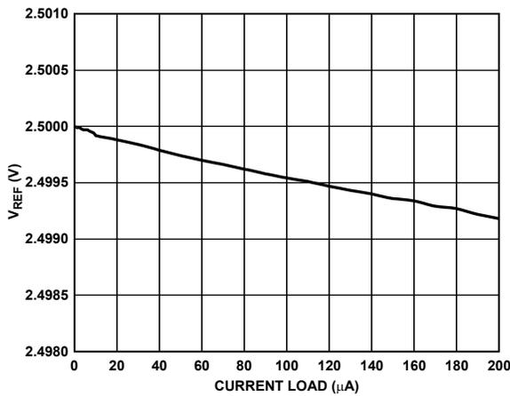
Figure 12.  $V_{REF}$  vs. Reference Output Current Drive
