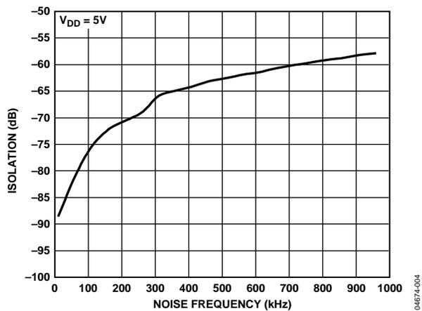
Figure 5. Channel-to-Channel Isolation
