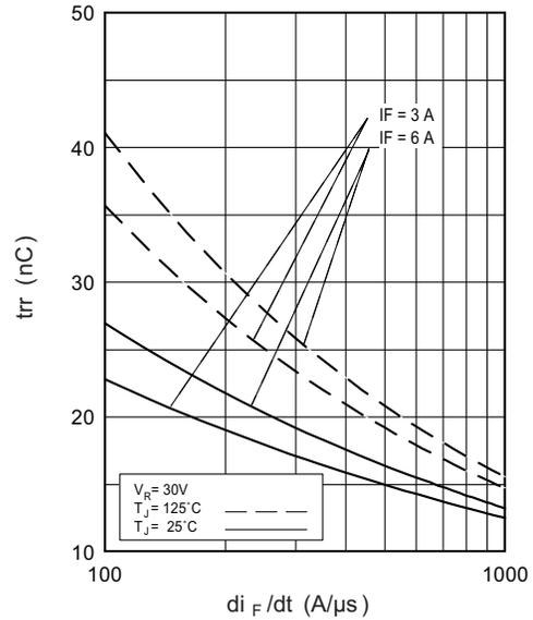
Fig. 7 - Typical Reverse Recovery vs.  $di_F/dt$
