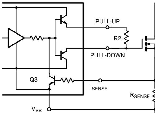
**Figure 6.** Simplified Peak Shoot-Through Current Limiting Circuit
