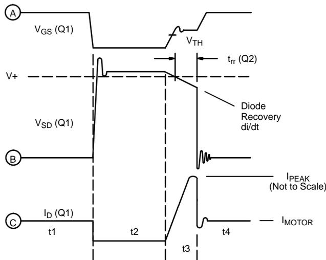
Figure 4. Controlling di/dt via MOSFET Gate Drive Impedance
