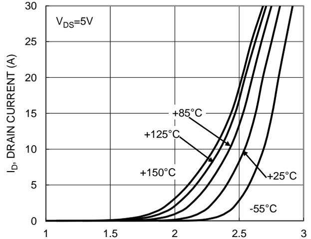
Figure 2. Typical Transfer Characteristic
