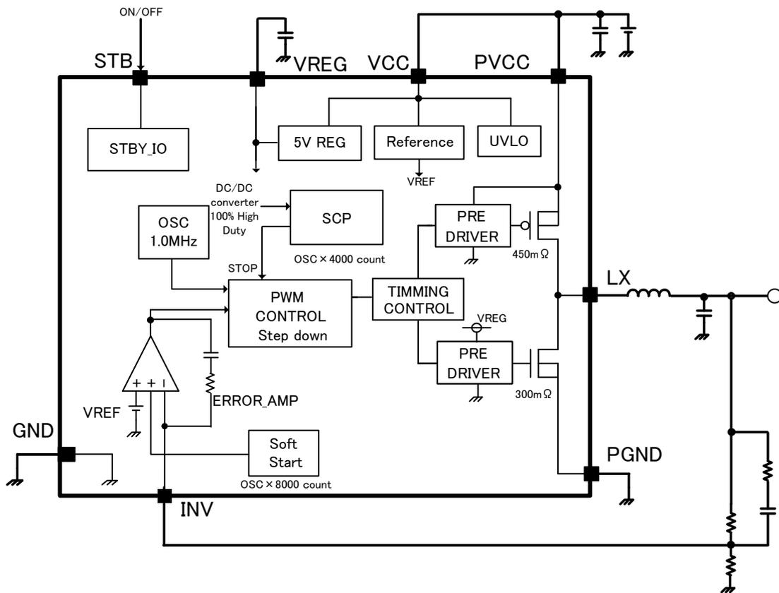
Fig.2 Block diagram
