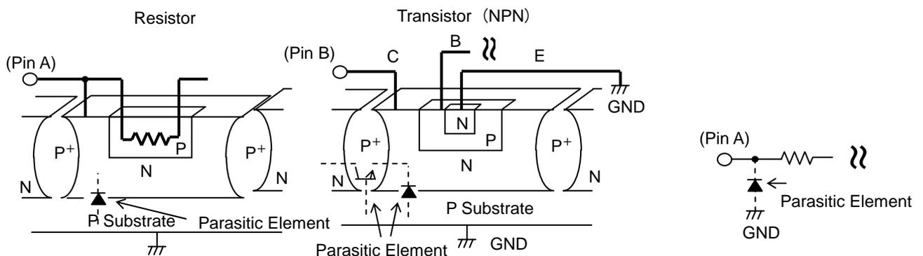
Fig.53 Example of simple structure of Bipolar IC
