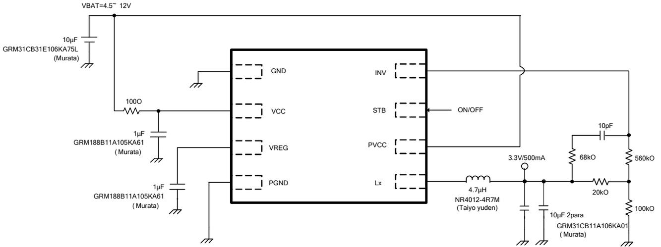
Fig.32 Reference application diagram2
