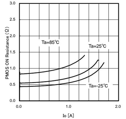
Fig.17. PchFET ON resistance Io property [VCC=5.0V]
