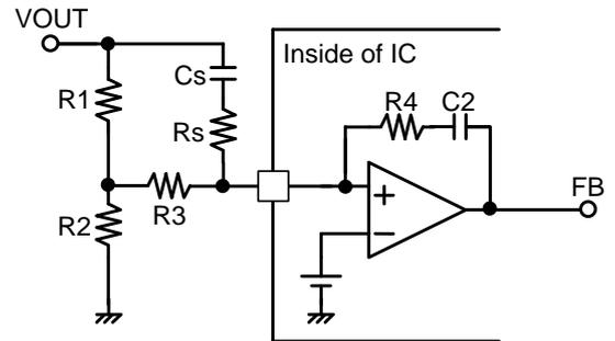
Fig.51 Example of phase compensation setting
