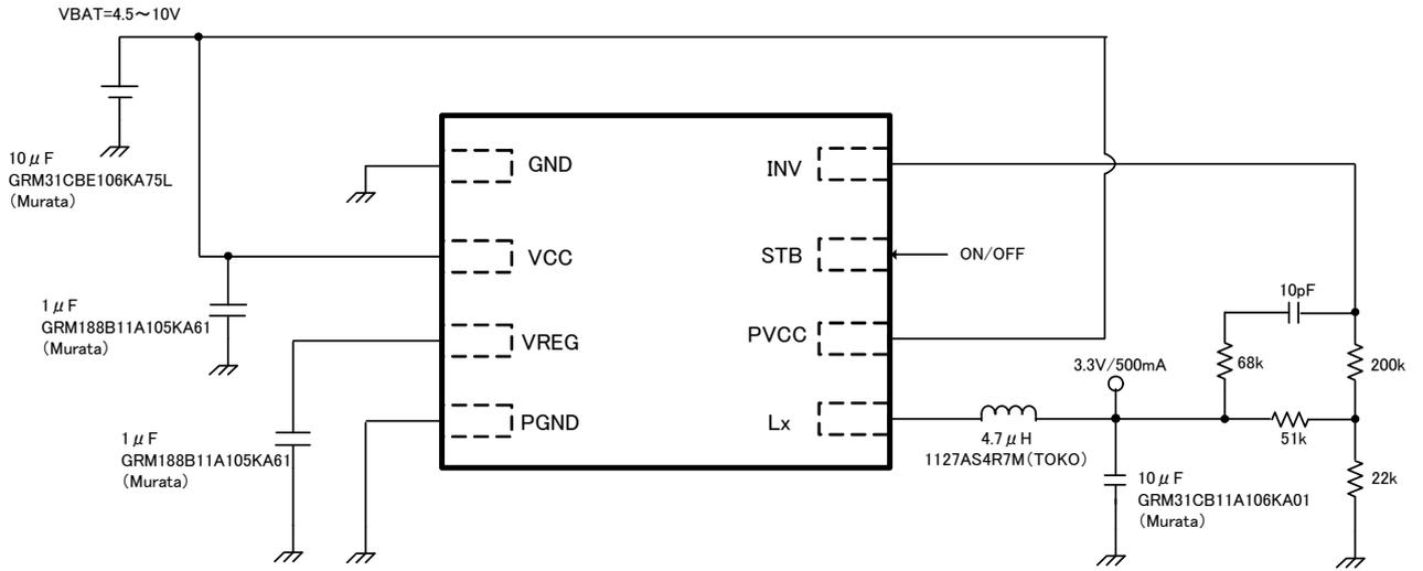
Fig.21 Reference application diagram1
