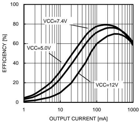
Fig.33 Power conversion efficiency (VOUT = 1.2 V)
