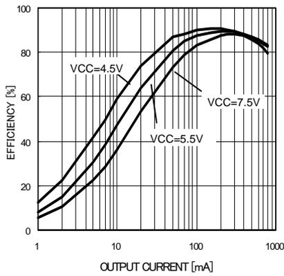
Fig.22 Power conversion efficiency (VOUT = 3.3 V)
