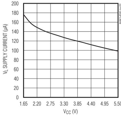
**$V_{CC}$  DYNAMIC SUPPLY CURRENT vs.  $V_L$  SUPPLY VOLTAGE (PUSH-PULL DRIVING ONE IOVL\_)**
