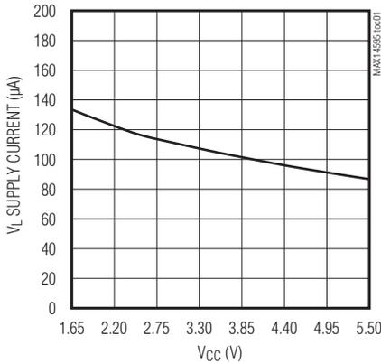
**$V_L$  DYNAMIC SUPPLY CURRENT vs.  $V_{CC}$  SUPPLY VOLTAGE (PUSH-PULL DRIVING ONE IOVCC\_)**
