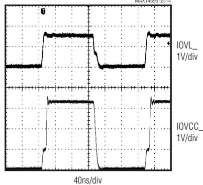
**RAIL-TO-RAIL DRIVING (OPEN-DRAIN DRIVING ONE IOVL<sub>-</sub>)**
