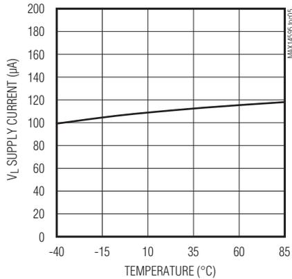
**$V_L$  DYNAMIC SUPPLY CURRENT vs. TEMPERATURE (PUSH-PULL DRIVING ONE IOVCC\_)**
