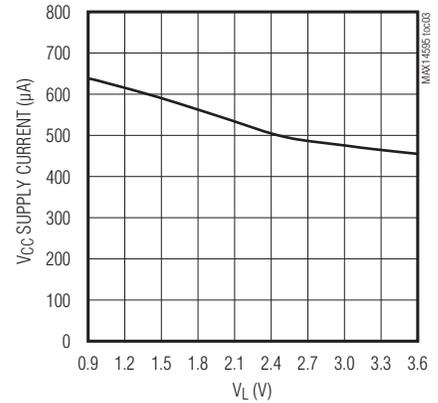
**$V_{CC}$  DYNAMIC SUPPLY CURRENT vs.  $V_L$  SUPPLY VOLTAGE (OPEN-DRAIN DRIVING ONE IOVCC\_)**
