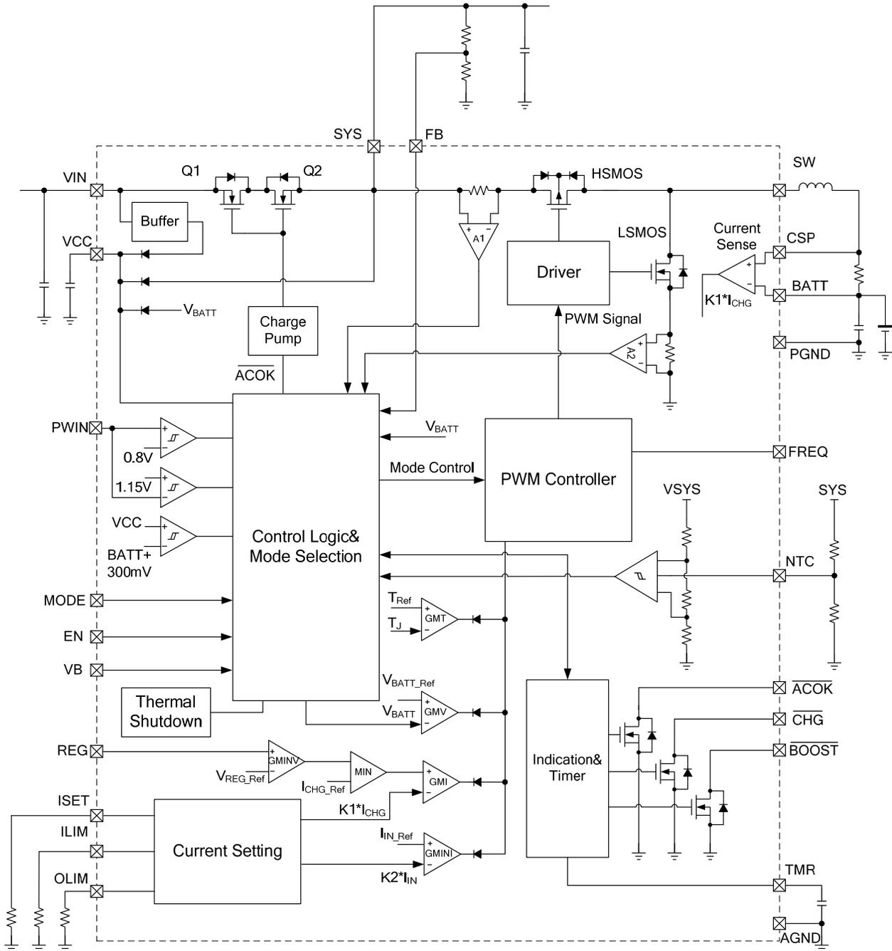
**Figure 1: Functional Block Diagram in Charge Mode**
