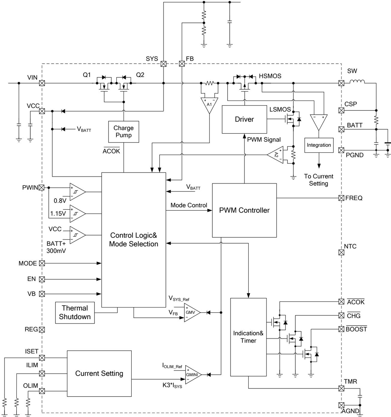
Figure 2: Functional Block Diagram in Boost Mode
