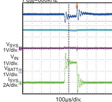
**Input Voltage Clamp @ 4.6V**
