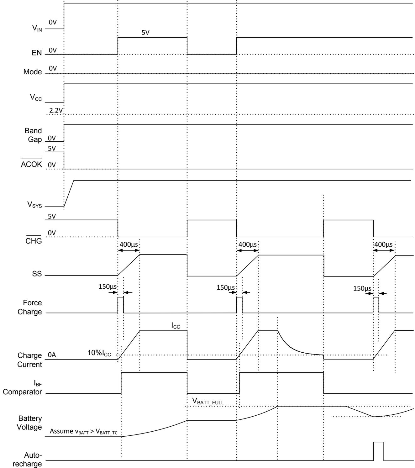
Figure 8: EN Start-Up Time Flow in Charge Mode
