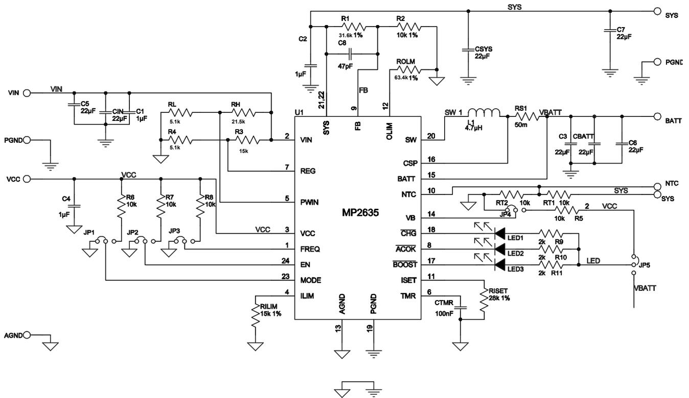
Figure 14: The detailed application circuit of MP2635
