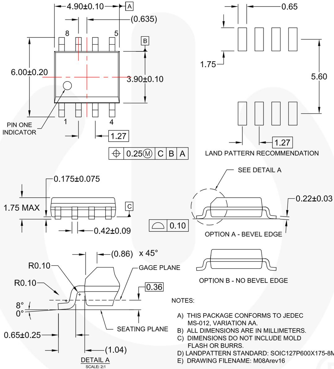
Figure 6. 8-LEAD, SOIC, JEDEC MS-012, 0.150" NARROW BODY
