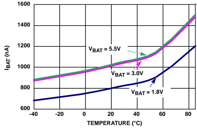
FIGURE 5.  $I_{BAT}$  vs TEMPERATURE ( $V_{DD} = 0V$ )
