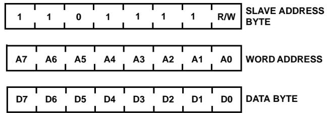
FIGURE 20. SLAVE ADDRESS, WORD ADDRESS, AND DATA BYTES
