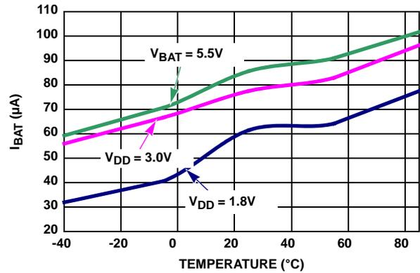
FIGURE 11. I<sub>BAT</sub> WITH TSE = 1, BTSE = 1 vs TEMPERATURE
