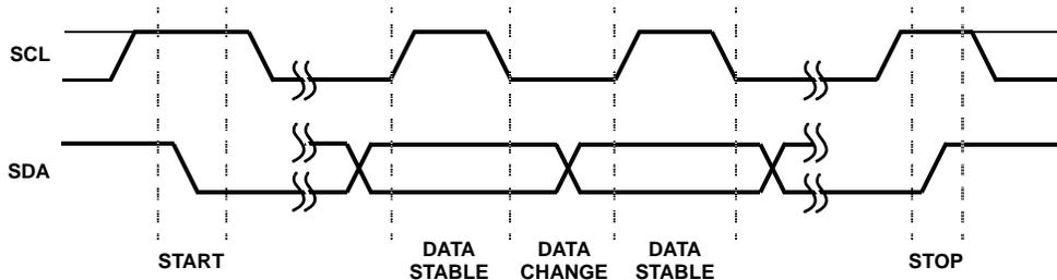
FIGURE 17. VALID DATA CHANGES, START AND STOP CONDITIONS
