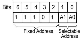
**Figure 21. Address Bit Definition for 7-Bit Address**
