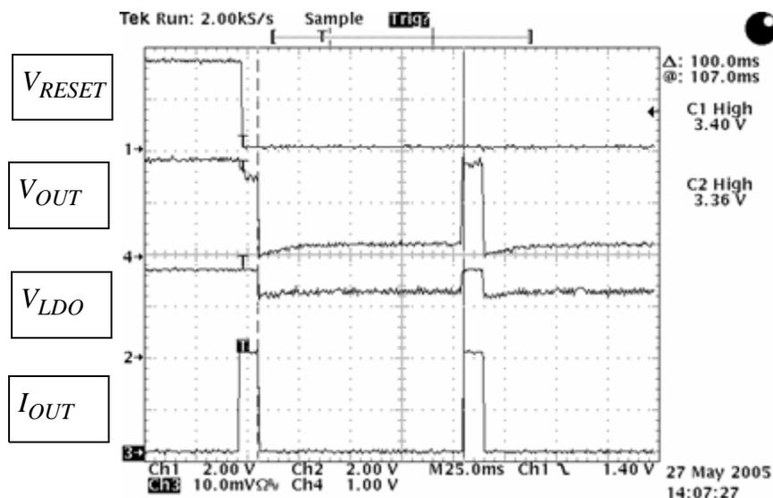
Figure 30. Buck is in the Over Current Condition
