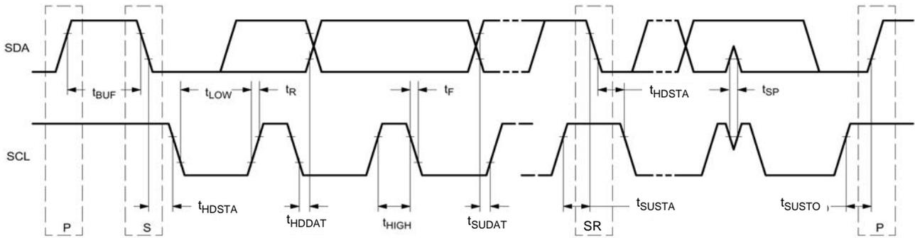
**Figure 4. Definition of Time on the I<sup>2</sup>C Bus**
