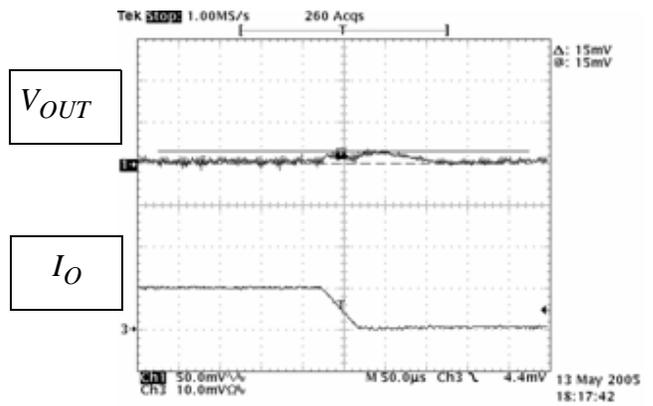
Figure 47. Load Transient Response
