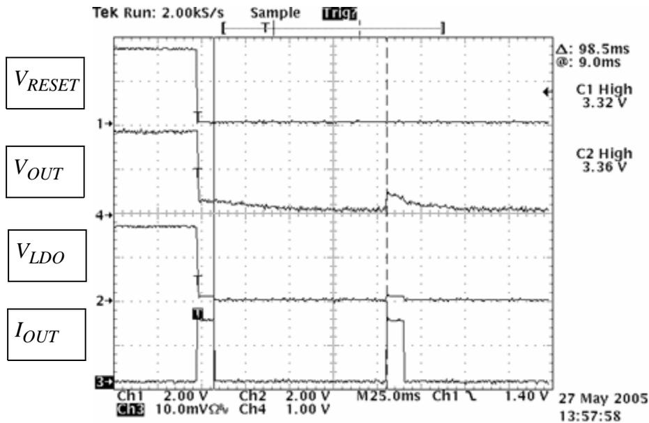
Figure 32. LDO in the Over Current Condition
