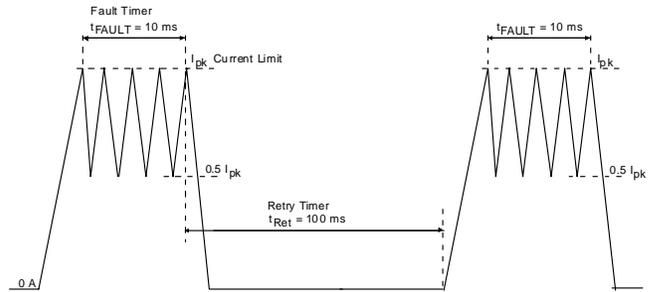
Figure 13. Switching Regulator Current Limit (Not To Scale)
