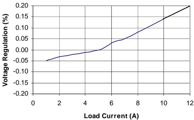
**Figure 7. Buck Converter Voltage Regulation vs Load Current**
