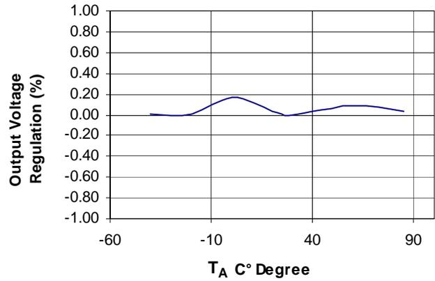
**Figure 8. Buck Converter Voltage Regulation vs Ambient Temperature**
