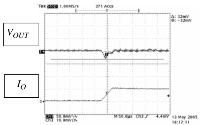
Figure 46. Load Transient Response
