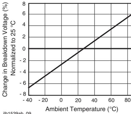
Fig. 10 - Switch Breakdown Voltage vs. Temperature
