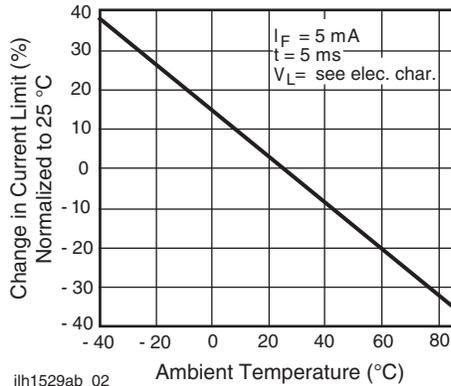
Fig. 3 - Current Limit vs. Temperature
