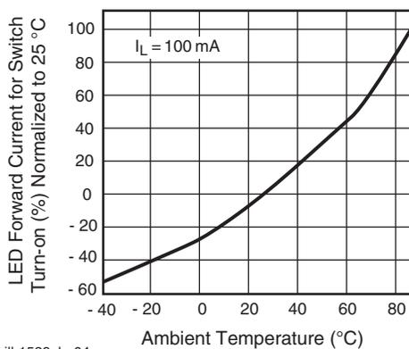
Fig. 5 - LED Current for Switch Turn-on vs. Temperature
