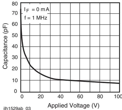
Fig. 4 - Switch Capacitance vs. Applied Voltage
