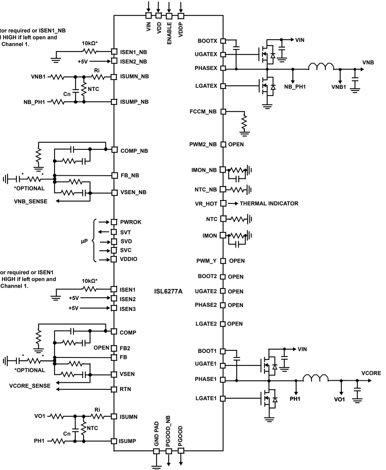
FIGURE 6. TYPICAL APPLICATION CIRCUIT USING INDUCTOR DCR SENSING
