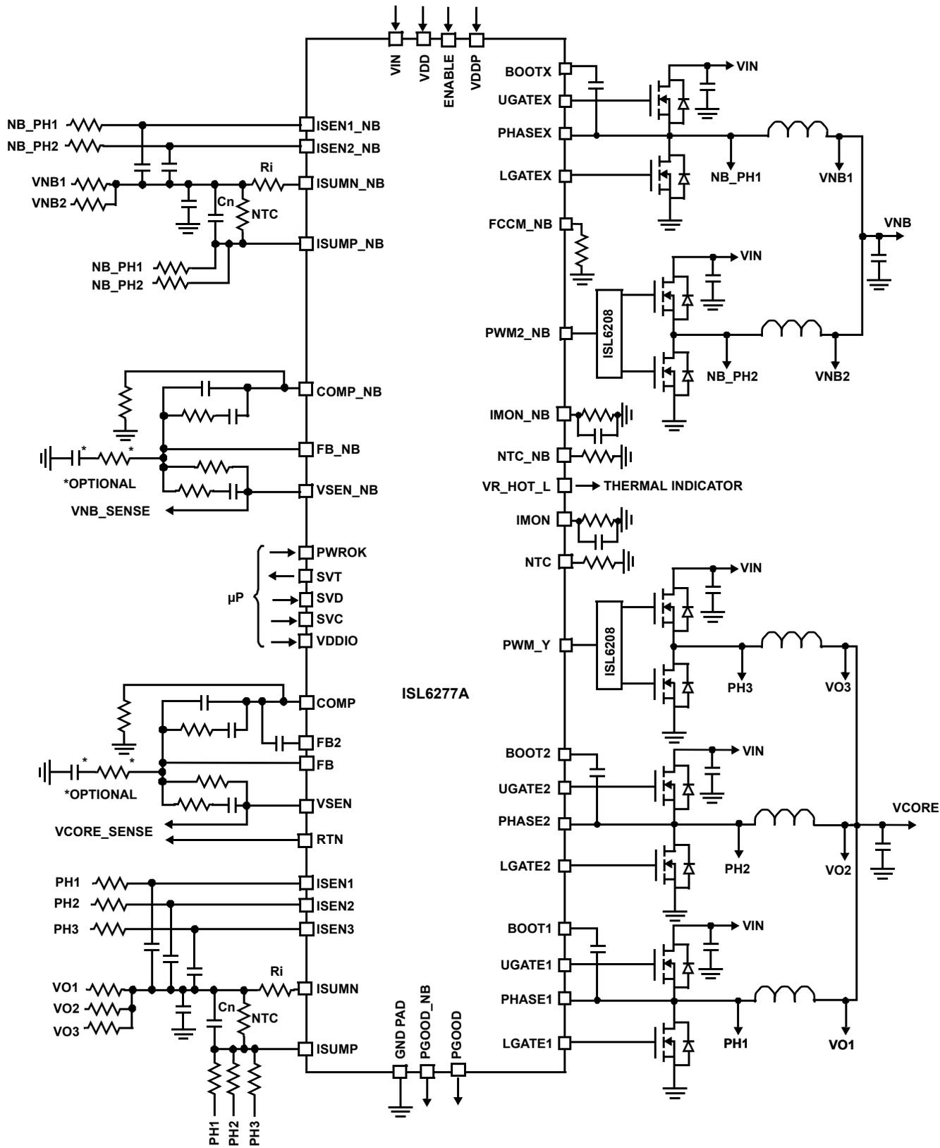
FIGURE 3. TYPICAL APPLICATION CIRCUIT USING INDUCTOR DCR SENSING
