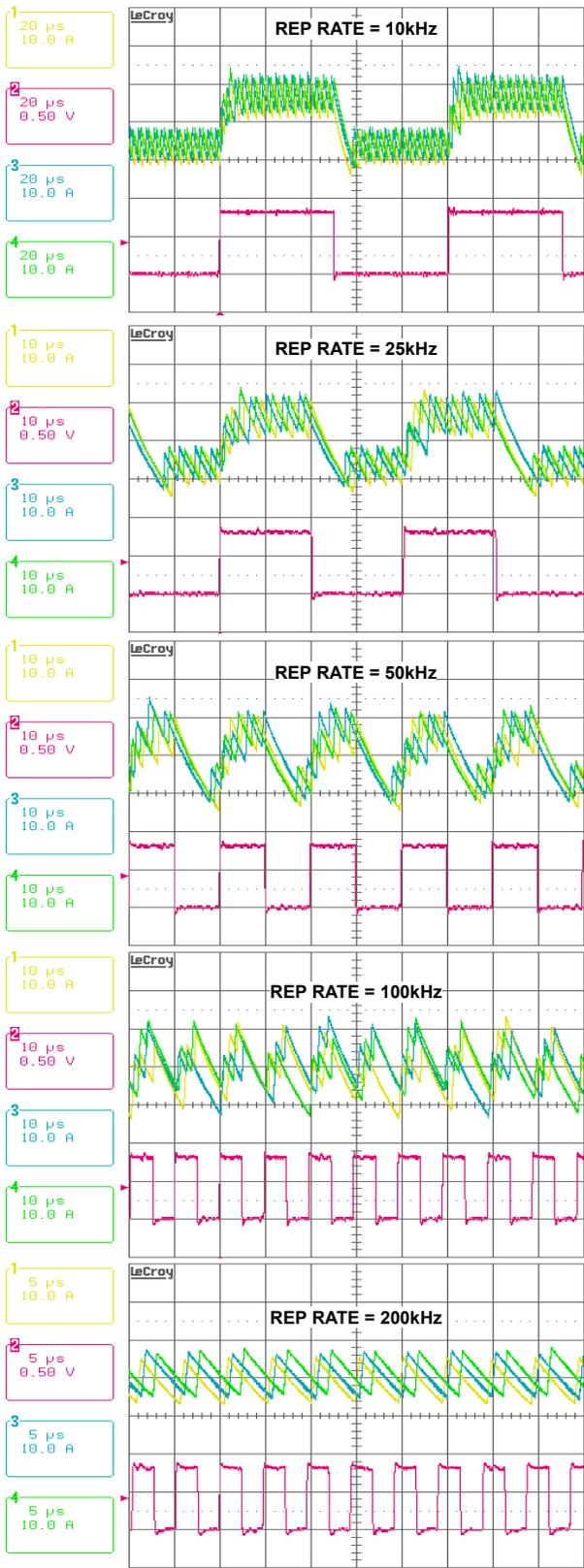
**FIGURE 19. CURRENT BALANCING DURING DYNAMIC OPERATION.**
