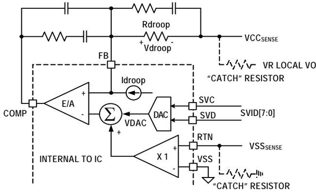
**FIGURE 16. DIFFERENTIAL SENSING AND LOAD LINE IMPLEMENTATION**
