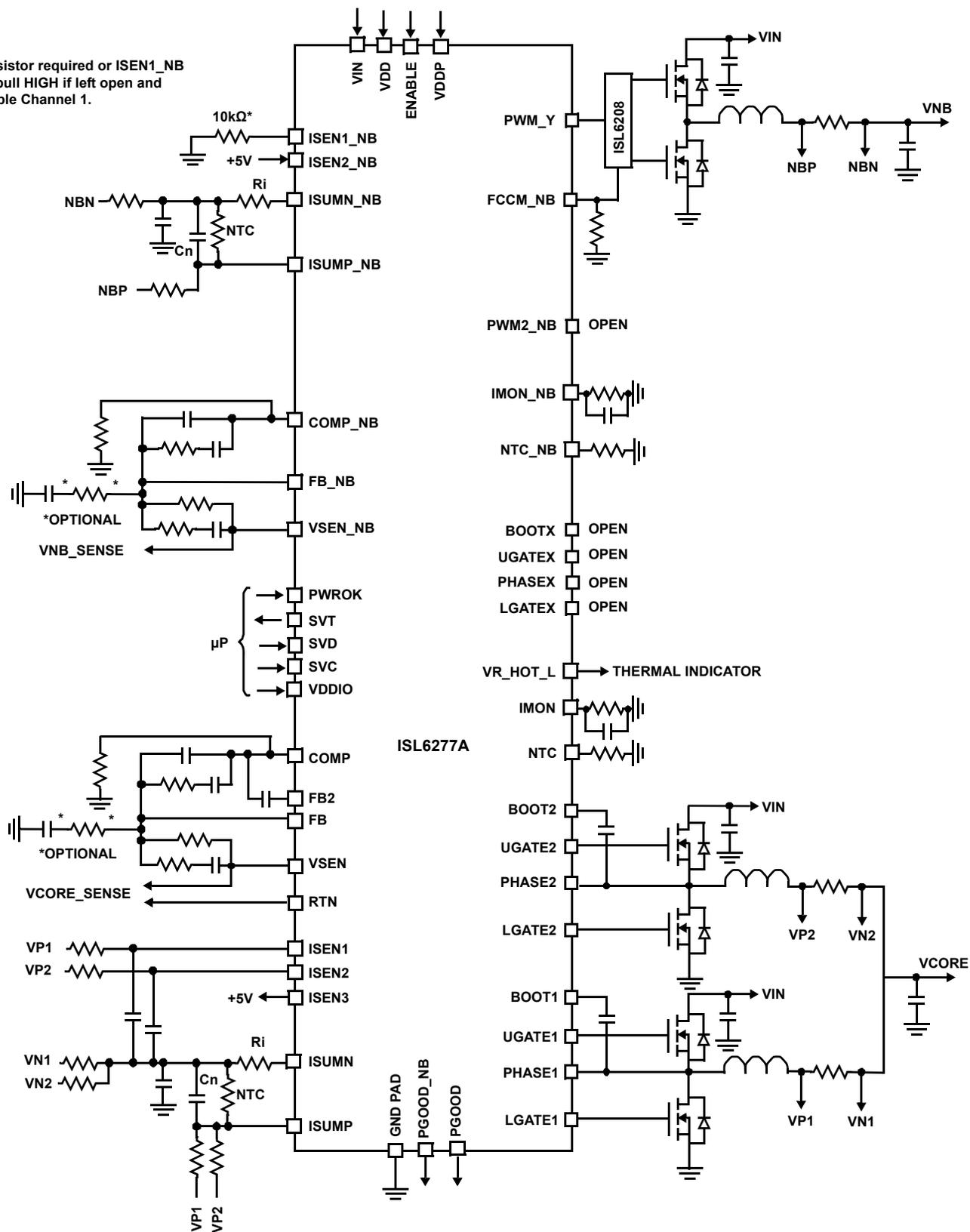
FIGURE 5. TYPICAL APPLICATION CIRCUIT USING RESISTOR SENSING
