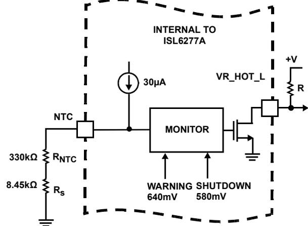
**FIGURE 34. THERMAL MONITOR FEATURE OF THE ISL6277A**
