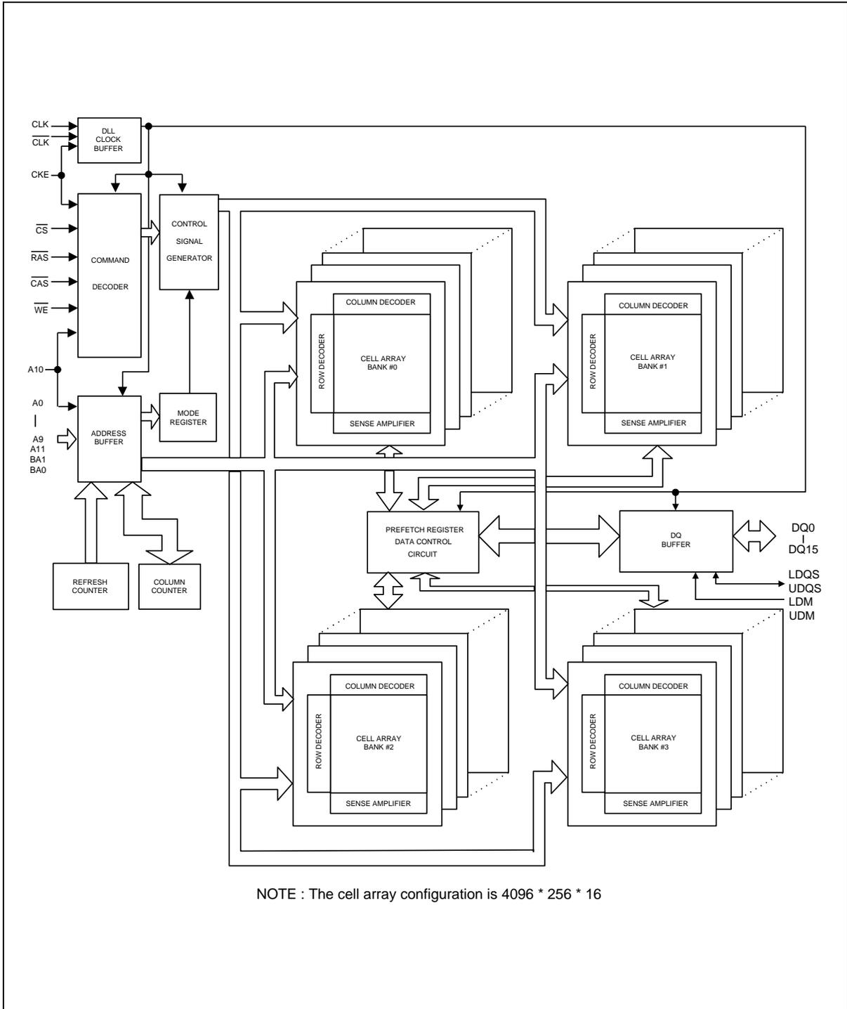
NOTE : The cell array configuration is 4096 \* 256 \* 16
