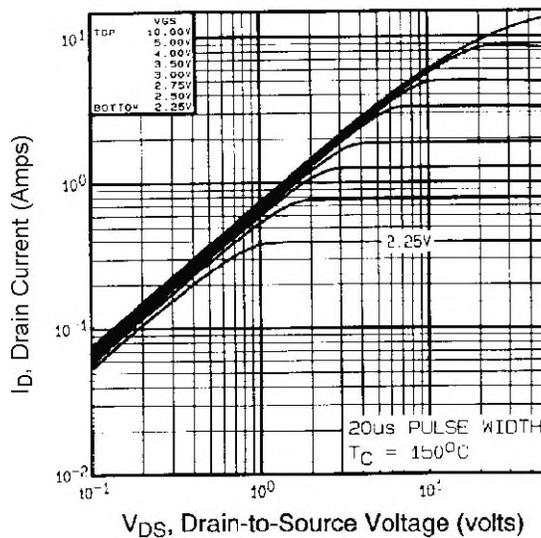
Fig. 2 - Typical Output Characteristics,  $T_C = 150^\circ\text{C}$
