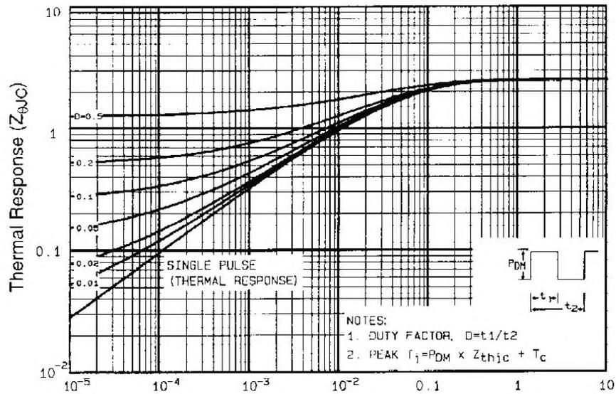
Fig. 11 - Maximum Effective Transient Thermal Impedance, Junction-to-Case
