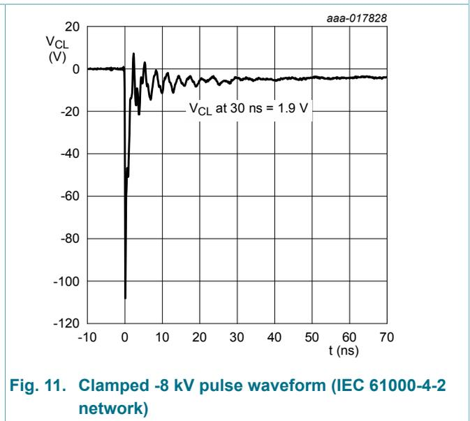
Fig. 11. Clamped -8 kV pulse waveform (IEC 61000-4-2 network)
