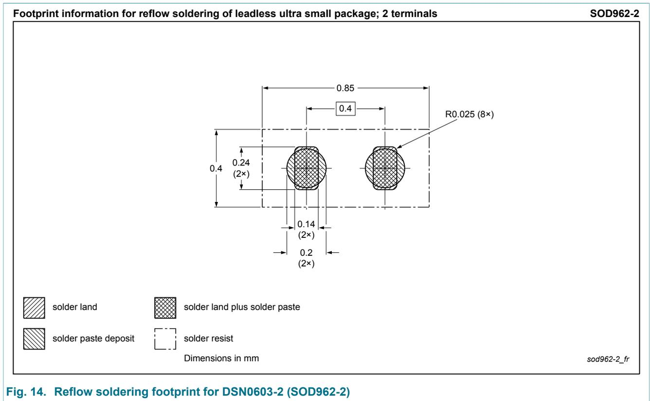
Fig. 14. Reflow soldering footprint for DSN0603-2 (SOD962-2)
