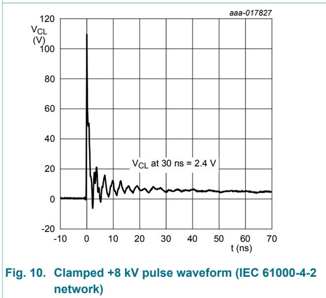
Fig. 10. Clamped +8 kV pulse waveform (IEC 61000-4-2 network)
