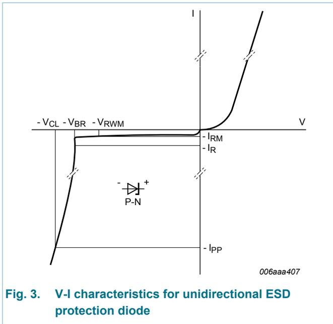
Fig. 3. V-I characteristics for unidirectional ESD protection diode
