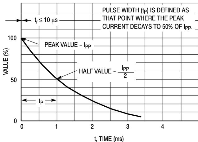
Figure 1.  $10 \times 1000 \mu\text{s}$  Pulse Waveform
