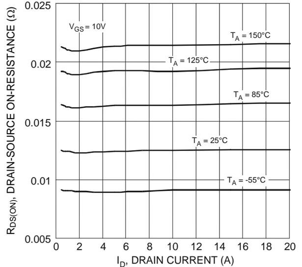
Figure 4 Typical On-Resistance vs. Drain Current and Temperature
