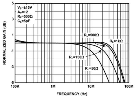
FIGURE 10. GAIN vs FREQUENCY FOR VARIOUS  $R_{LOAD}$  ( $A_V = +2$ )
