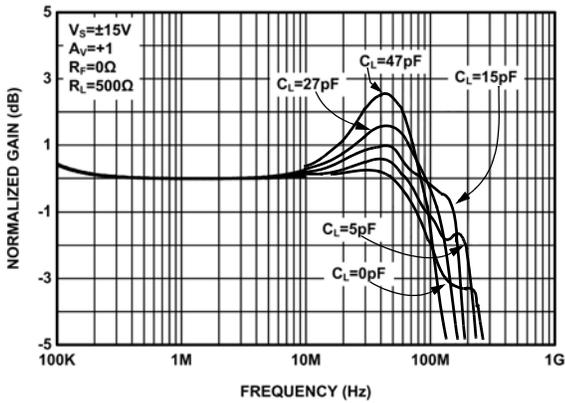
FIGURE 11. GAIN vs FREQUENCY FOR VARIOUS  $C_{LOAD}$  ( $A_V = +1$ )
