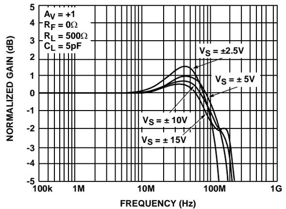
FIGURE 16. GAIN vs FREQUENCY FOR VARIOUS SUPPLY SETTINGS
