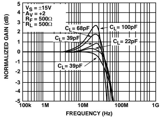
FIGURE 12. GAIN vs FREQUENCY FOR VARIOUS  $C_{LOAD}$  ( $A_V = +2$ )
