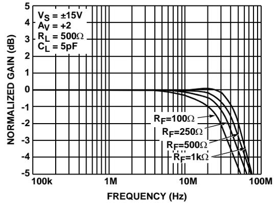
FIGURE 14. GAIN vs FREQUENCY FOR VARIOUS  $R_{FEEDBACK}$  ( $A_V = +2$ )
