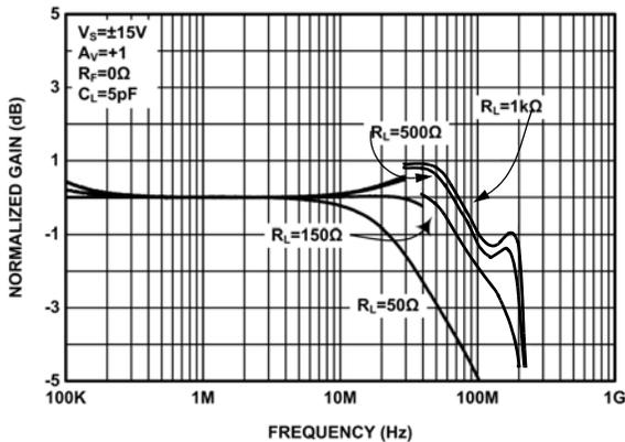
FIGURE 9. GAIN vs FREQUENCY FOR VARIOUS  $R_{LOAD}$  ( $A_V = +1$ )
