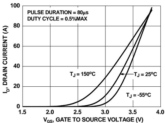
Figure 5. Transfer Characteristics
