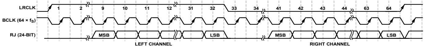
Figure 71. Right Justified (RJ) Mode, 24 Bits per Channel
