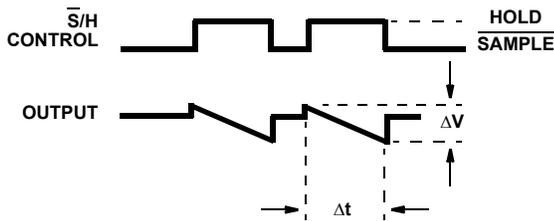
NOTE: Measure the slope of the output during hold,  $\Delta V/\Delta t$ , and compute drift current from:  $I_D = C_H \Delta V/\Delta t$ .
