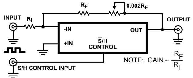
FIGURE 6. INVERTING CONFIGURATION
