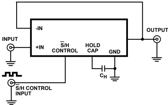
FIGURE 1. HOLD STEP ERROR AND DRIFT CURRENT
