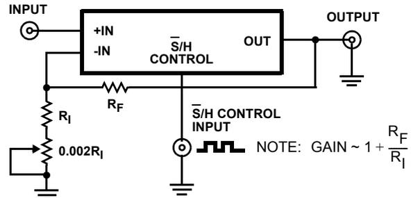
FIGURE 7. NON-INVERTING CONFIGURATION
