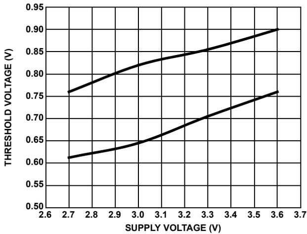
FIGURE 23. LOGIC INPUT THRESHOLD VOLTAGE vs SUPPLY VOLTAGE
