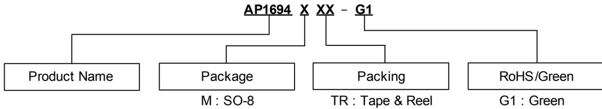
Diodes IC's Pb-free products with "G1" suffix in the part number, are RoHS compliant and green.
