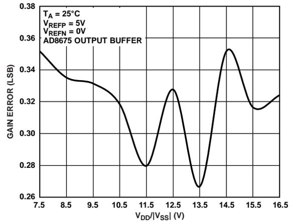
Figure 26. Gain Error vs. Supply Voltage, 5 V Span
