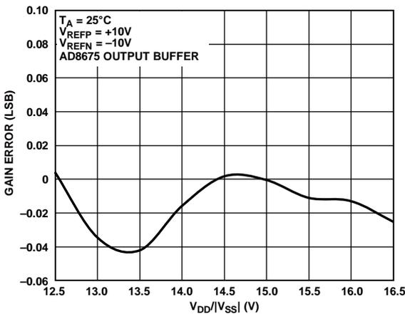
Figure 25. Gain Error vs. Supply Voltage, ±10 V Span
