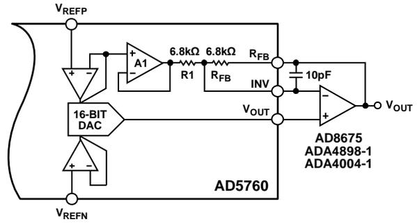
Figure 52. Output Amplifier in Gain of Two Configuration
