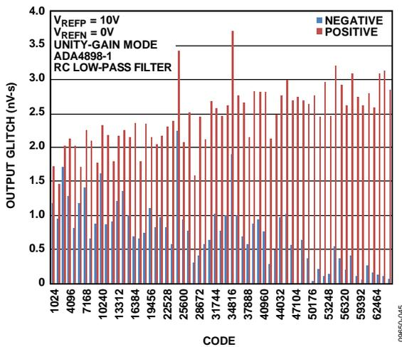
Figure 43. 6 MSB Segment Glitch Energy for 10V  $V_{REF}$
