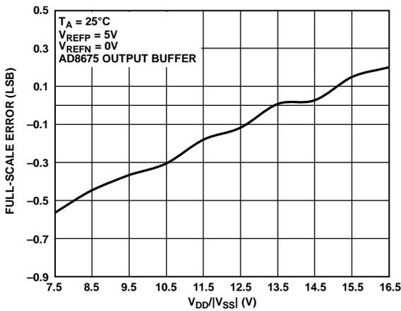
Figure 24. Full-Scale Error vs. Supply Voltage, 5 V Span
