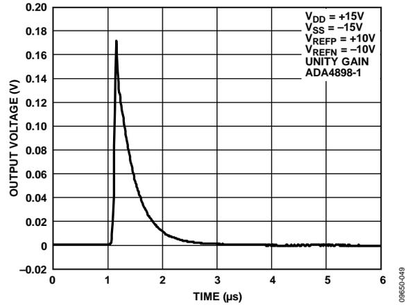
Figure 48. Glitch Impulse on Removal of Output Clamp
