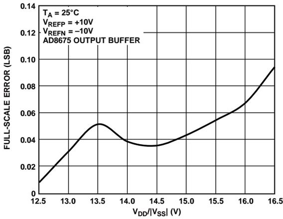
Figure 23. Full-Scale Error vs. Supply Voltage, ±10 V Span
