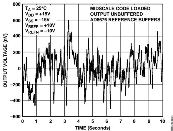
Figure 46. Voltage Output Noise, 0.1 Hz to 10 Hz Bandwidth
