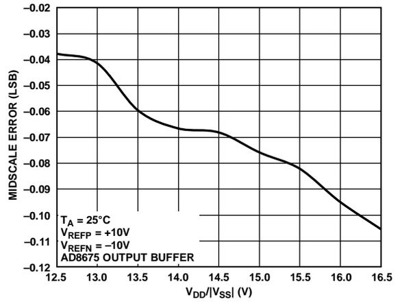
Figure 21. Midscale Error vs. Supply Voltage, ±10 V Span
