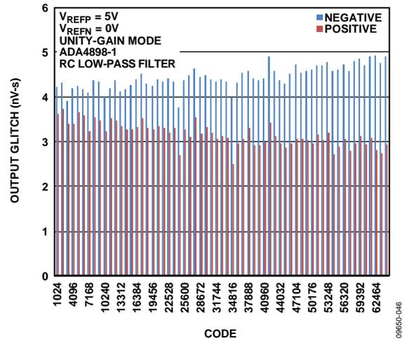
Figure 44. 6 MSB Segment Glitch Energy for 5V  $V_{REF}$
