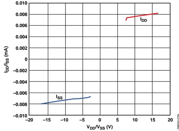
Figure 38. Power Supply Currents vs. Power Supply Voltages
