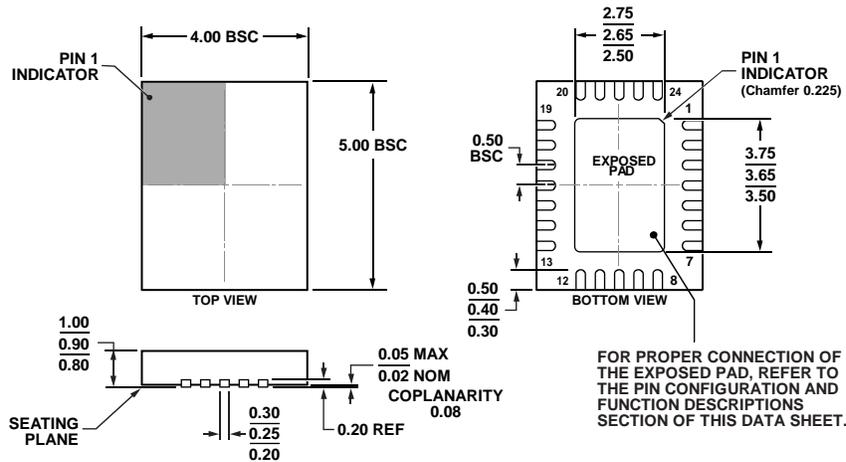
Figure 54. 24-Lead Lead Frame Chip Scale Package [LFCSP\_VQ]
