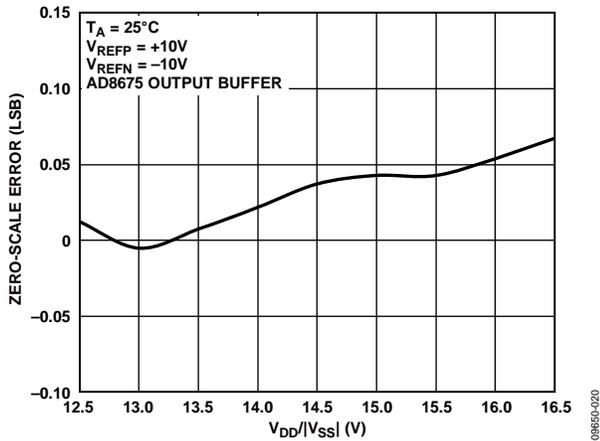
Figure 19. Zero-Scale Error vs. Supply Voltage, ±10 V Span
