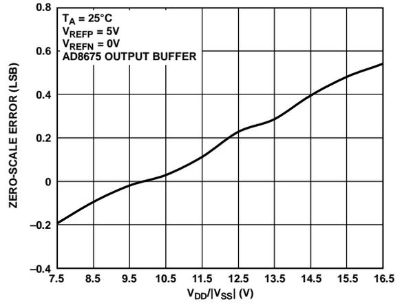
Figure 20. Zero-Scale Error vs. Supply Voltage, 5 V Span
