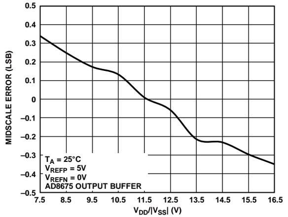
Figure 22. Midscale Error vs. Supply Voltage, 5 V Span
