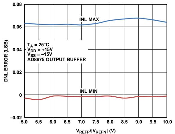
Figure 28. Differential Nonlinearity Error vs. Reference Voltage
