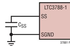
**Figure 5. Using the SS Pin to Program Soft-Start**
