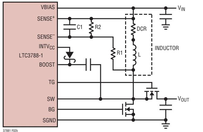
PLACE C1 NEAR SENSE PINS  $(R1 \parallel R2) \cdot C1 = \frac{L}{DCR}$   $R_{SENSE(EQ)} = DCR \cdot \frac{R2}{R1 + R2}$
