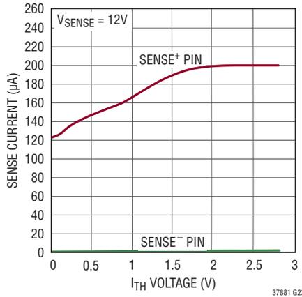
**SENSE Pin Input Current vs V<sub>SENSE</sub> Voltage**
