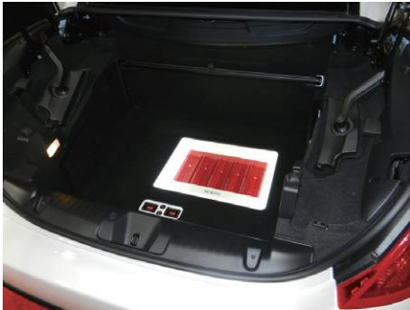
**Fig. 1 Power amplifier in Peugeot 308CC trunk**
