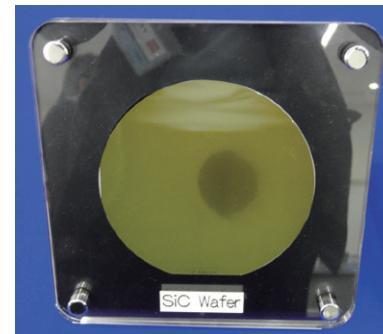
**Fig.1 Large diameter SiC wafers**
