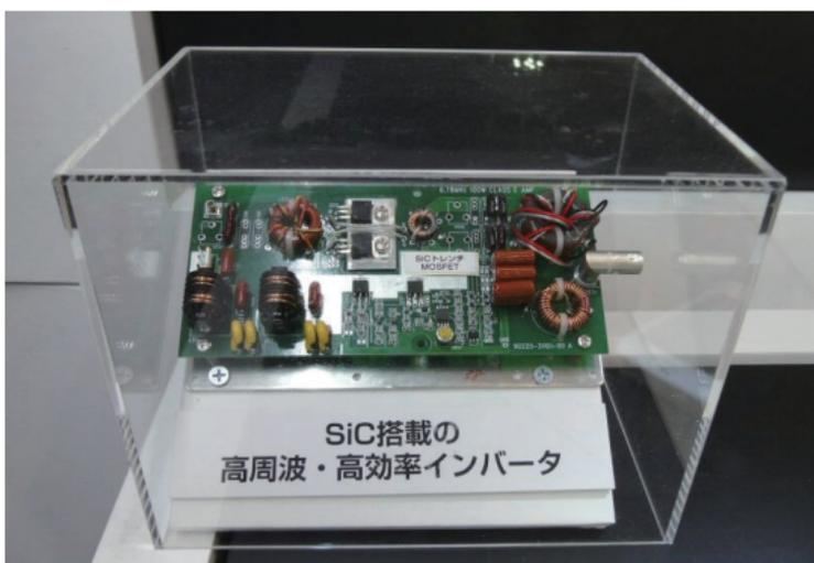
**Fig. 3 Wireless power supply system inverter**
