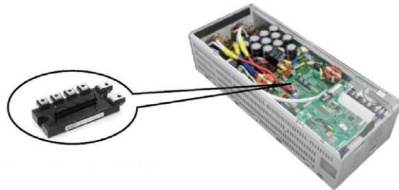
**Fig. 1 Power conditioner for photovoltaic systems**
