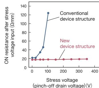
**Fig. 2 Suppressing current collapse**
