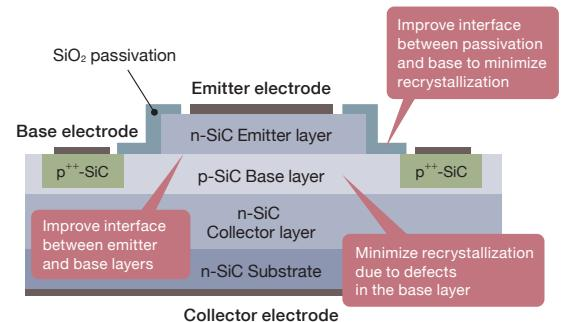
**Fig. 2 Boosting current amplification ratio with three major improvements**
