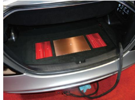
**Fig. 2 Power amplifier in trunk of Mercedes-Benz SLR McLaren Roadster**
