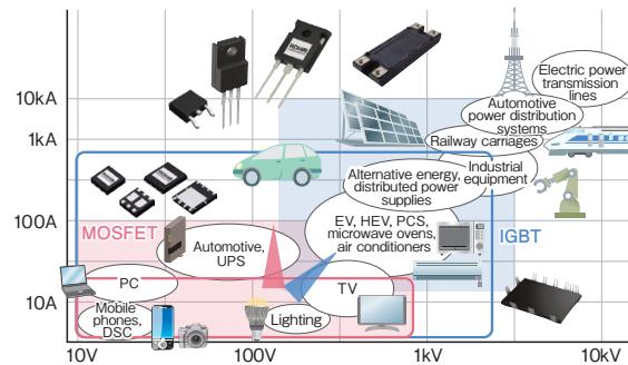
Fig. 1 ● Expanding range of application for power devices
