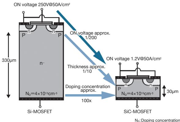
**Fig. 1 Slashing ON resistance**
