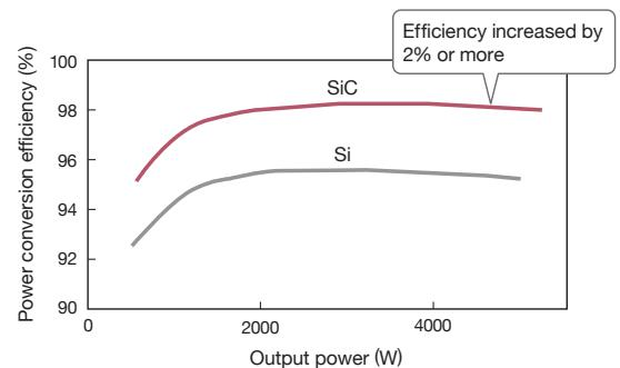
**Fig. 2 98% conversion efficiency**
