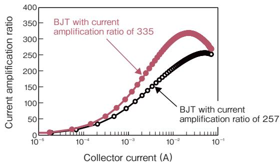
**Fig. 1 Current amplification ratio over 200**
