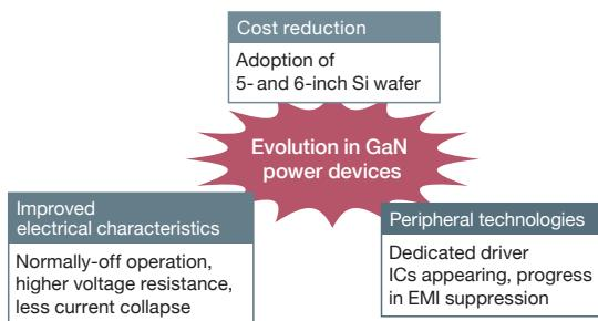
**Fig. 1 Resolving GaN power device issues**
