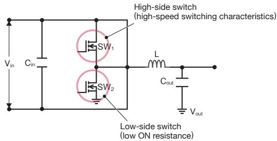
**Fig. 1 Power device configuration in DC-DC converter**
