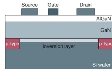
**Fig. 4 Suppressing leakage current to boost voltage resistance**
