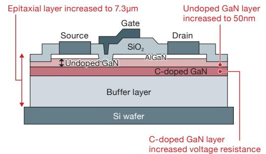
**Fig. 3 Attaining a 1.7kV voltage resistance**
