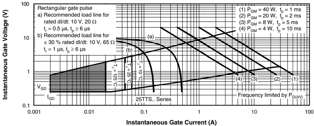
Fig. 8 - Gate Characteristics
