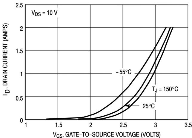
Figure 1. Transfer Characteristics
