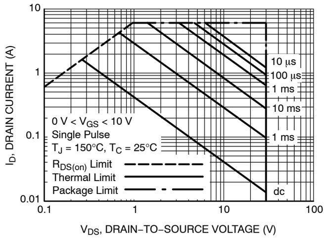
**Figure 9. Maximum Rated Forward Biased Safe Operating Area**
