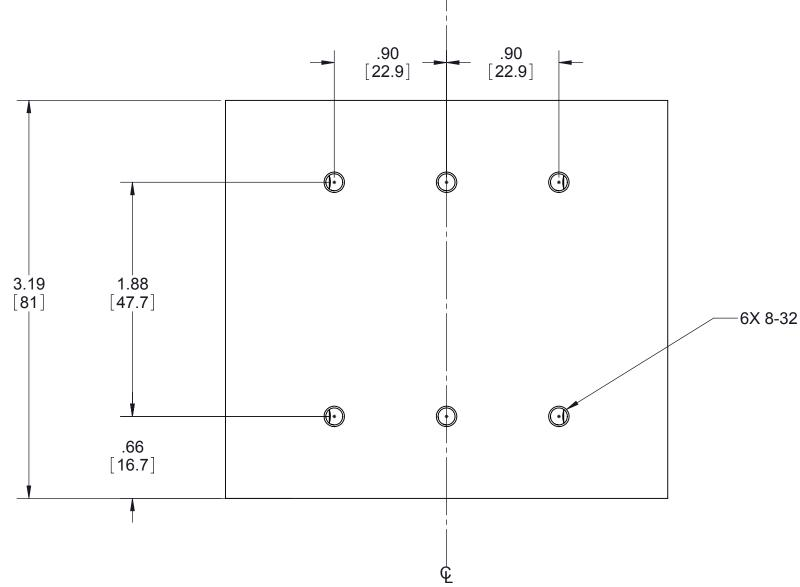
Tolerances: ± 0.02 in / 0.5 mm. All dimensions are in: inches [millimeters]
