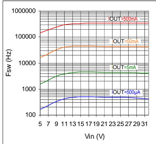
Figure 9. Average Switching Frequency vs.  $I_{OUT}$  ( $ILIM=open$ )
