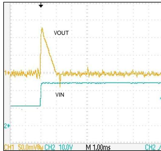
Figure 15. Line Regulation  $V_{OUT}=5V @ 10mA$
