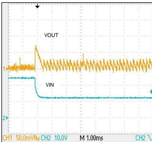
Figure 16. Load Regulation  $V_{OUT}=5V 10mA \rightarrow 500mA$
