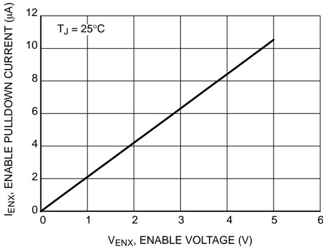
Figure 5. Enable Pulldown Current vs. Enable Voltage
