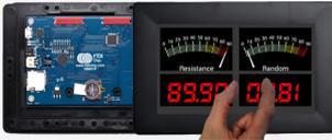
The VM800P and VM801P 'Plus' modules further extend system integration by providing a complete video subsystem with an embedded microcontroller in resistive touch and capacitive multitouch variants. In addition to the features supplied with the basic modules, this system provide an in-built MCU, the ATMEGA328P, which is supported by the Arduino libraries.
