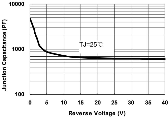
Fig.1-Typical Junction Capacitance
