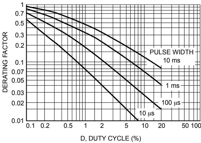
Figure 5. Typical Derating Factor for Duty Cycle
