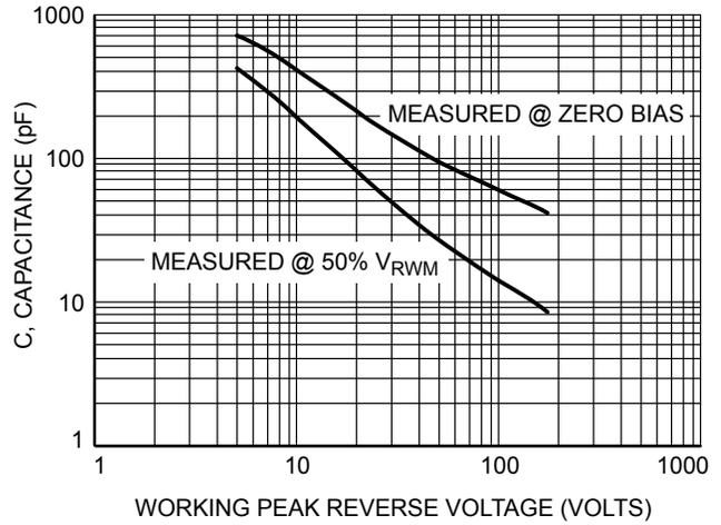
Figure 8. Capacitance versus Working Peak Reverse Voltage
