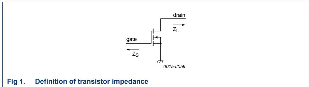
Fig 1. Definition of transistor impedance
