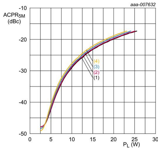
$V_{DS} = 28\text{ V}$ ;  $I_{Dq} = 224\text{ mA}$ ; carrier spacing = 5 MHz;  $f_c = 960\text{ MHz}$
