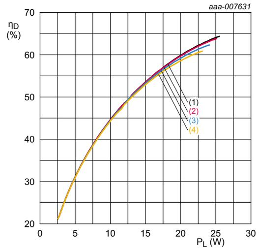
$V_{DS} = 28\text{ V}$ ;  $I_{Dq} = 224\text{ mA}$ ; carrier spacing = 5 MHz;
