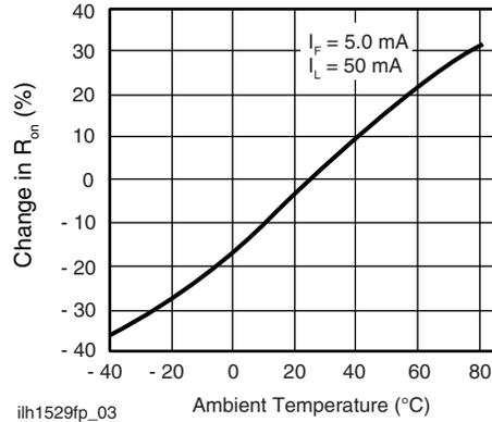
Fig. 3 - On-Resistance vs. Temperature
