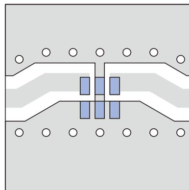
Line width should be designed to match 50Ω characteristic impedance, depending on PCB material and thickness.
