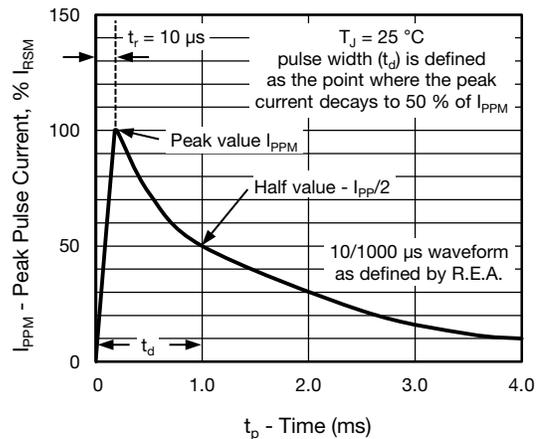
Fig. 3 - Pulse Waveform
