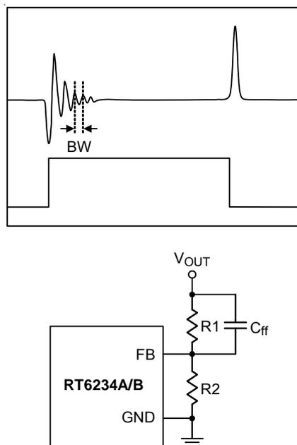
Figure 1. C<sub>ff</sub> Capacitor Setting
