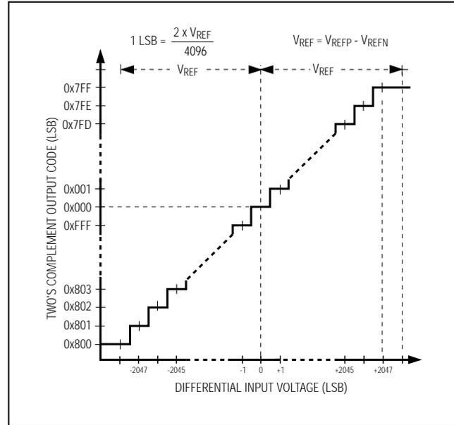
Figure 6. Two's Complement Transfer Function ( $G/\bar{T} = 0$ )
