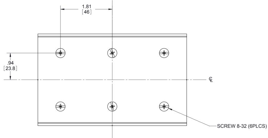
Tolerances: ± 0.02 in / 0.5 mm. All dimensions are in: inches [millimeters]
