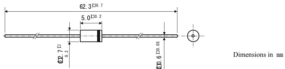
\*1 The allowance position of Body against the center of whole lead wire is 0.5mm(max.)
