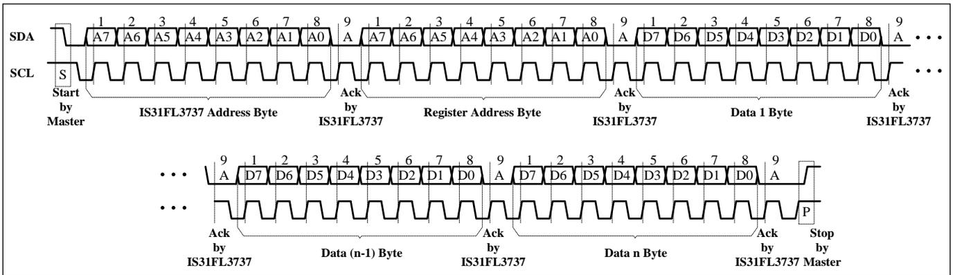
Figure 7 Writing to IS31FL3737 (Automatic address increment)
