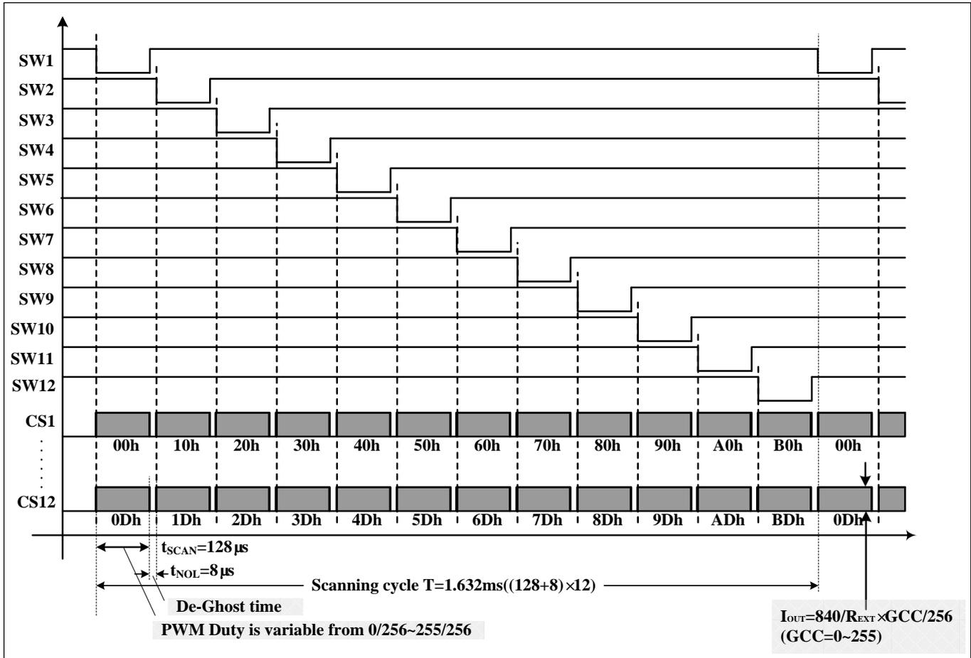
Figure 12 Scanning Timing
