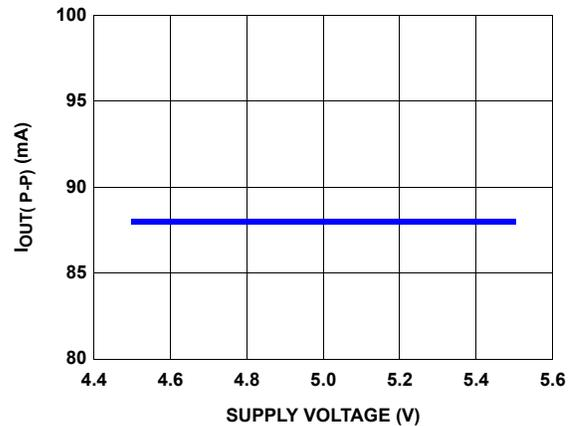
FIGURE 12. PEAK-TO-PEAK OUTPUT CURRENT vs SUPPLY VOLTAGE
