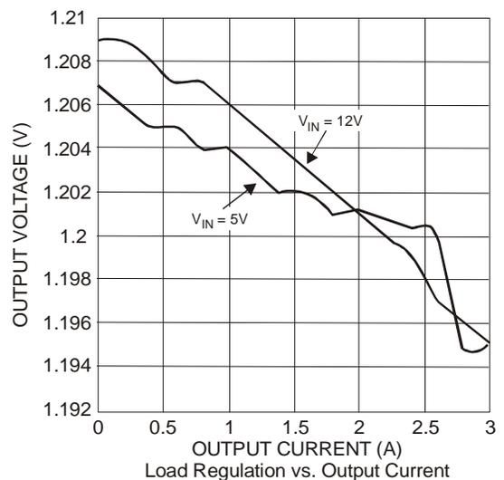
**Typical Performance Graphs (cont.) ( $V_{IN} = 12V$ ,  $V_{OUT} = 1.2V$ ,  $T_A = +25^\circ C$ , unless otherwise noted)**
