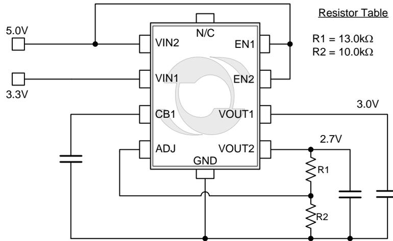
**Figure 1 – Fixed / Adjustable Output Application**
