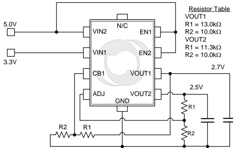
**Figure 2 – Adjustable / Adjustable Output Application**
