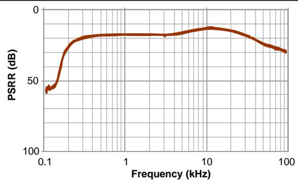
Typical performance characteristics, unless otherwise specified are:  $C_{IN} = C_{OUT} = 1\mu F$ ,  $C_{BY} = 470pF$ ,  $V_{IN} = V_{OUT} = 2.5V$ ,  $T_A = 25^\circ C$ , ENABLE is tied to  $V_{IN}$ .
