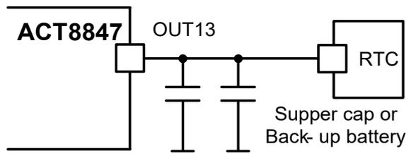
REG13 features a constant current-limit, which protects the IC under output short-circuit conditions as well as provides a constant charge current, when operating as a backup battery charger.
